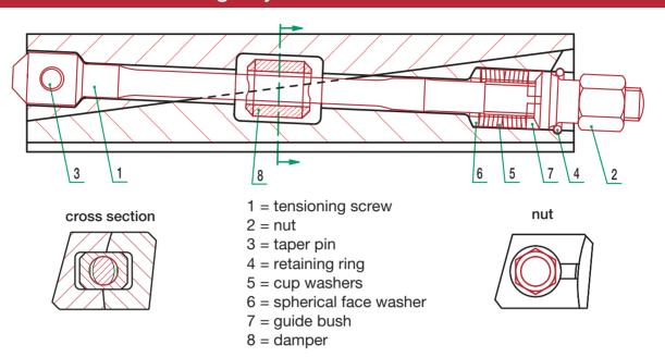
On the Feuerbacher tensioning keys "D" the tendency for vertical offsetting of the Feuerbacher tensioning key halves is taken up by a damping block. This is particularly valuable when clamping upper dies.
