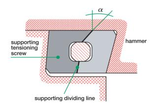
The Feuerbacher tensioning keys version "SB" have a fully supporting contact face and a supporting clamping screw providing a significantly improved clamping effect.
